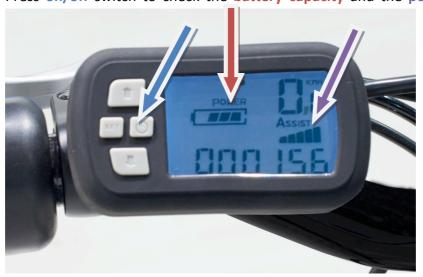
1.9 To avoid dangerous unplanned acceleration, always make sure that the electrical system is turned off and the power indicator is not illuminated when mounting, dismounting or leaving the bike unattended. For your safety, turn off the battery power switch when stopped or walking the bike
