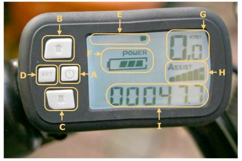
Battery capacity. Three bars indicate 80% capacity left, two bars indicate 70% left, one 55% capacity left, half bar 5% capacity left.
