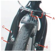
A-Cable clamp bolt C-pad fixing bolt E-Arm fixing bolt E-Arm fixing bolt
