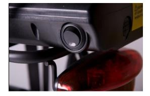
2.1.8 Press the **on/off** switch (labeled with O' symbol) on the LCD display, located on the left hand side of the handlebars. Check the **battery capacity** and the **power assistance level** selected.
