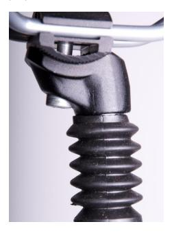
IMPORTANT - never raise the saddle past the point where the maximum marks on the saddle post are visible above the quick release colla, r and never grease the seatpost.
