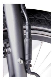
3.12.2 Remove the single Allen screw, securing the motor cable clamp to the front fork (shown above) and the protective covers on the front wheel spindle nuts.
