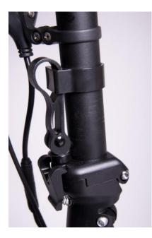
Then release the quick release clamp, located on the cross bar, and swing the clamp through 90 degrees around a vertical axis. Then push vertically down on the plunger assembly to uncouple the two halves of the folding locking mechanism and fold the two halves of the bike together.
