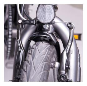
3.7.4 Squeeze both brake arms together and unhook the curved tubular cable guide end from the left hand brake arm (as viewed from the front of the bike in the above image). This will allow the brake arms to spring clear of the wheel rim. Use a 5mm Allen key to loosen the bolts holding the brake pads to the arms (right and left), then take the spacers and washers out.
