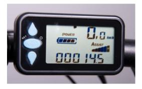
3.4.3 80%, 90% and 100% mode are generally used when you need a greater amount of assistance from the motor. 60% mode is used when you do not need the instant power of 90% or 100%. 40% and 50% are used in high traffic situations or poor conditions such as ice and snow when 80%, 90% and 100% power immediately could be dangerous.
