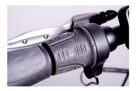
3.5.2 The independent use of the throttle, when available, will enable you to use the throttle without pedaling. However to achieve optimum performance and life from the motor, it is recommended that opening the throttle fully from standing still should be avoided, and that's where possible pedal assistance should be used when starting the bike from rest.
