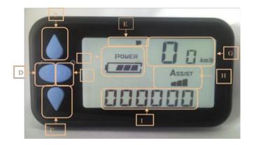
3.2.2 When the ON/OFF button is pushed and held for three seconds, and the capacity indicator goes out, you have turned the bike "off". When the bike is "off", you will not get any assistance from the battery and motor - the bike is effectively an unpowered pushbike. To turn the power back on, so the pedelec and throttle work again, simply press the ON/OFF button once - the capacity indicator will illuminate showing the power is on.
