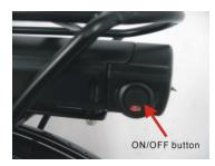
the on/off button on the battery to on. To turn off the bikes electrical system, switch the on/off button to off. (Please refer to the adjacent picture)
