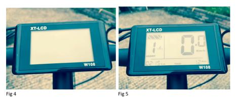
2.1.9 To avoid unplanned acceleration, always make sure that the LCD assist level is set to 0 when mounting, dismounting and turn the bike off when leaving it unattended.
