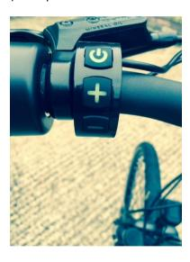
When the on/off button is pressed for 3 seconds the LCD symbols will become visible. When the on/off button is pushed again for 3 seconds, the LCD symbols will disappear - you have turned the bike "off". When the bike is "off" you will not get any assistance from the battery and motor and the bike is effectively an unpowered pushbike.
