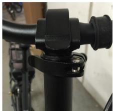
3.7.3 To alter the height of the handle bars, slacken clamp at the front of the stem. Slide the handle bars to the requires position and securely clamp into position making sure there is no movement in the clamp or handle bar stem.
