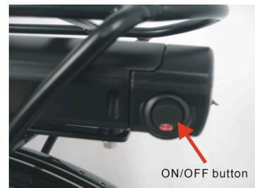
9.3 After the battery has been turned on the bike is ready for use. The battery box capacity indicator is on the handle bar for ease of use. Assistance from the battery is then available.
