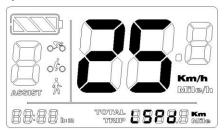
Attention: the speed limit unit is Km/h, which only works for 1-3 modes, sport mode , the speed limit do not work.
