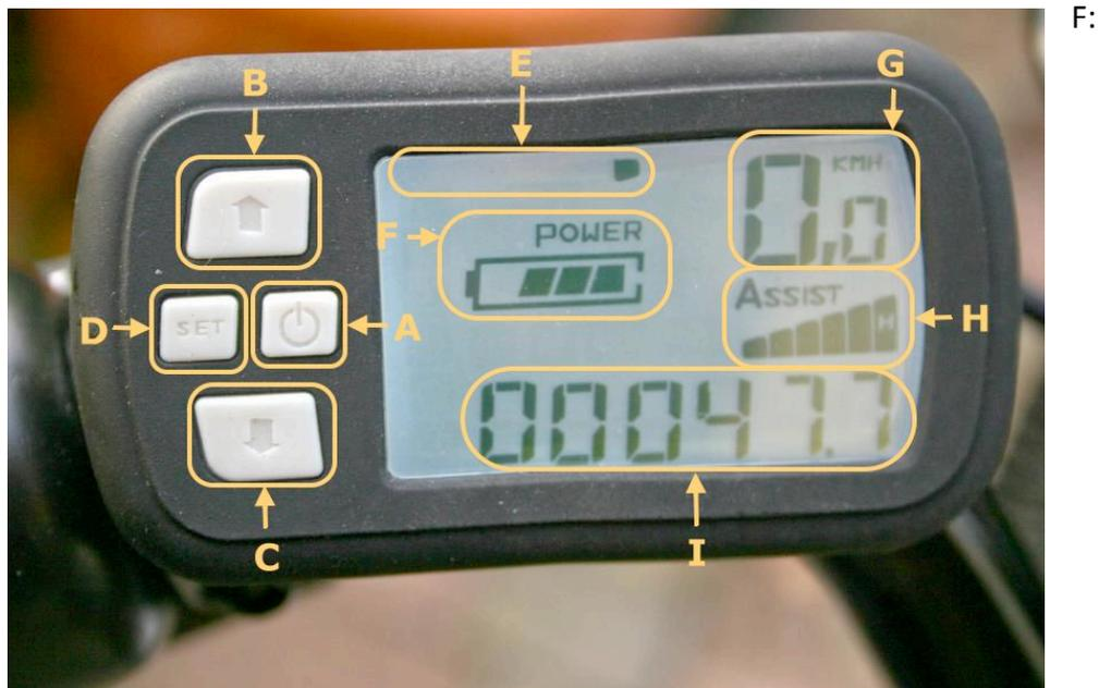
Battery capacity. Three bars indicate 80% capacity left, two bars indicate 70% left, one 55% capacity left, half bar 5% capacity left.
