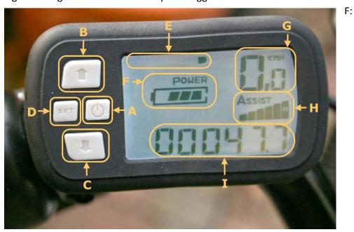
Battery capacity. Three rhombus left means 80% capacity left, two rhombus left means 70% left, one rhombus means 55% capacity left, half rhombus means 5% capacity left.
