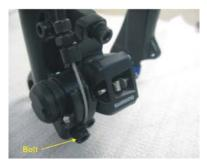
14.3.1.3. Adjust the cable adjuster bolt on the caliper So that there is 0.3mm clearance between the outside pad and the rotor. Turn this bolt toward clockwise direction means more clearance, anti-clockwise means less clearance.
