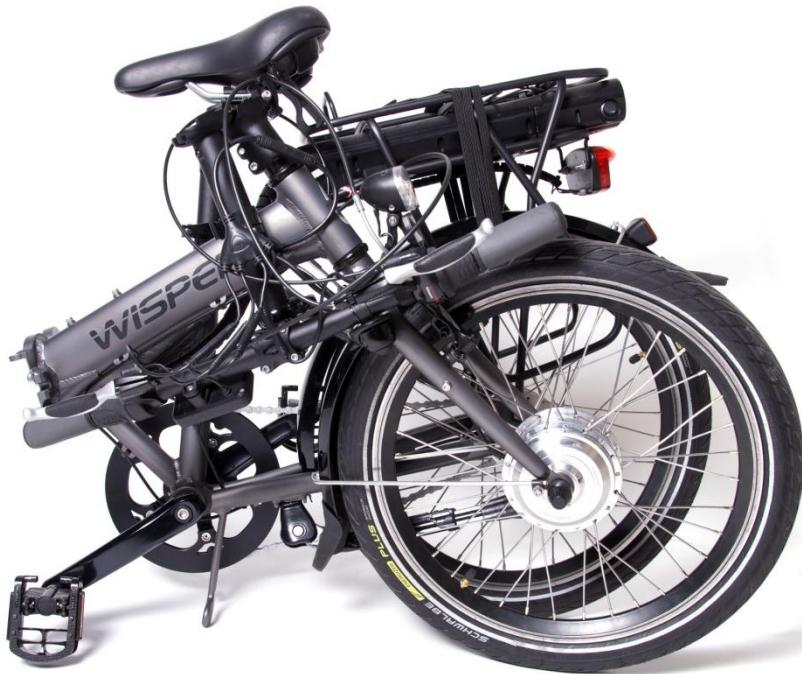
3.9.6 To unfold the bike, follow the reverse steps above ensuring all quick release clamps are securely fastened and no cables are trapped. Ensure the safety catch for the handlebar lower quick release lever is engaged after making the adjustment. Also ensure the stainless spring cable protector is in place.
