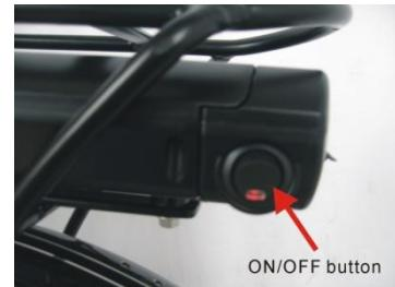
3.9.3 After the battery has been turned on the bike is ready for use. There is a battery capacity indicator on the battery and on the LCD handle bar LCD display. Press and hold the battery indicator button on the battery to check the capacity LEDs. All lights should be displayed on a fully charged battery.
