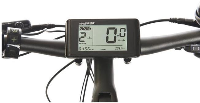
2.1.9 To avoid unplanned acceleration, always make sure that the LCD assist level is set to 0 when mounting, dismounting and turn the bike off when leaving it unattended.
